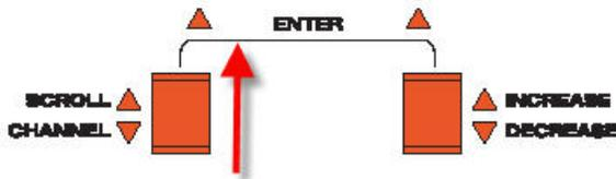
3. Press the SCROLL button up until "MDL" appears on the screen.
